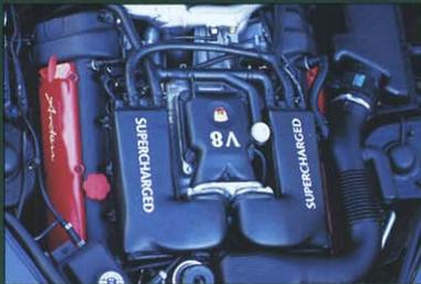
Arden high performance engine with 460 hp / 339 kW and 620 Nm torque
