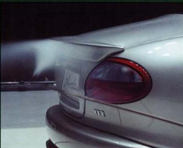
Arden rear spoiler in the wind tunnel test
